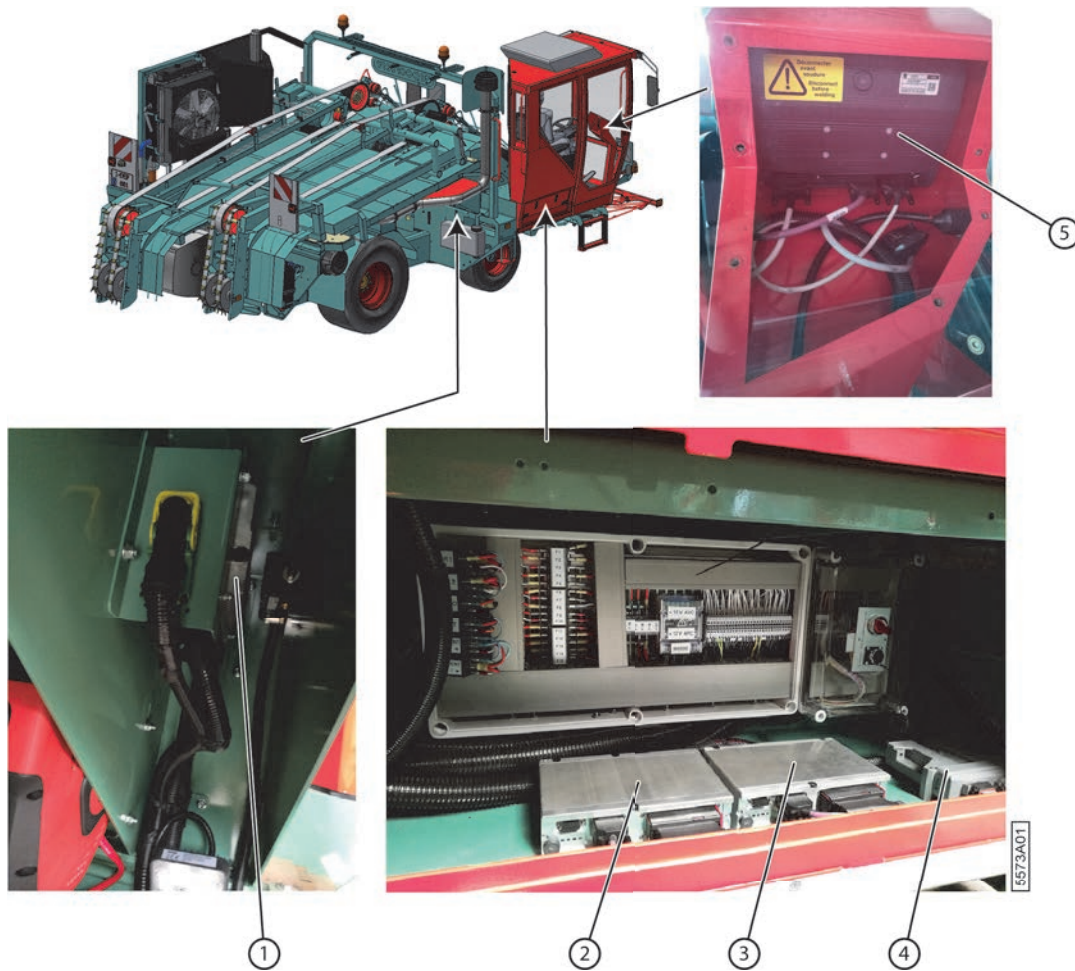
Fig. 168: The location of the controllers
