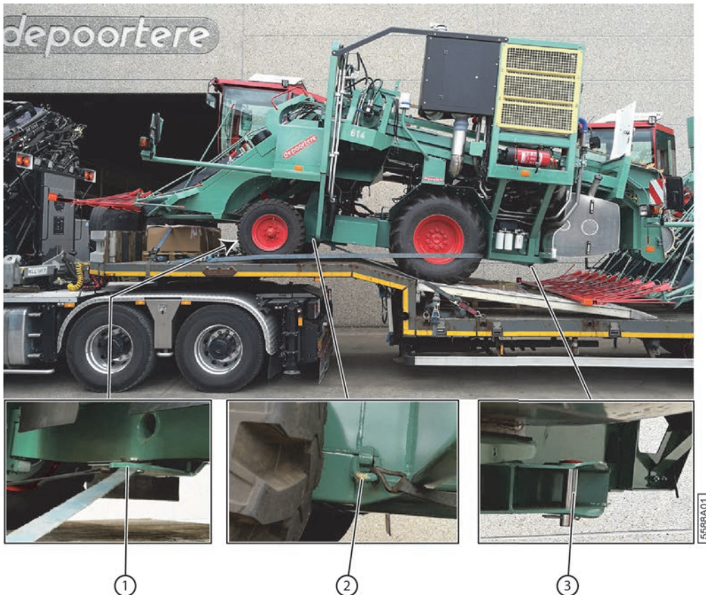
Fig. 47: Unloading the machine from the lorry (preparation)
