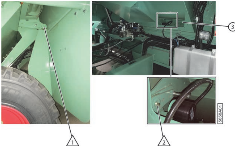
Fig. 140: Lubricating the pivot points of the picking element
