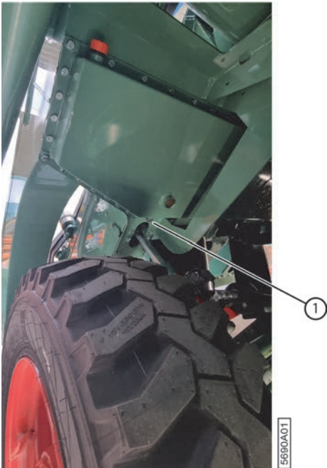
Fig. 109: Draining oil gearbox picking element
