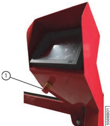
Fig. 44: Location of the emergency stop button
