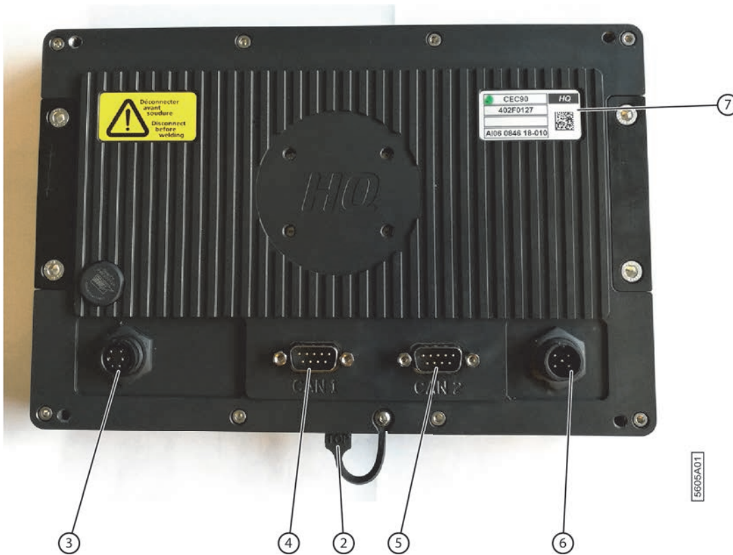
Fig. 61: The control screen (rear)
