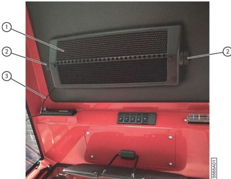
Fig. 19: Air conditioning system (bluetooth version)
