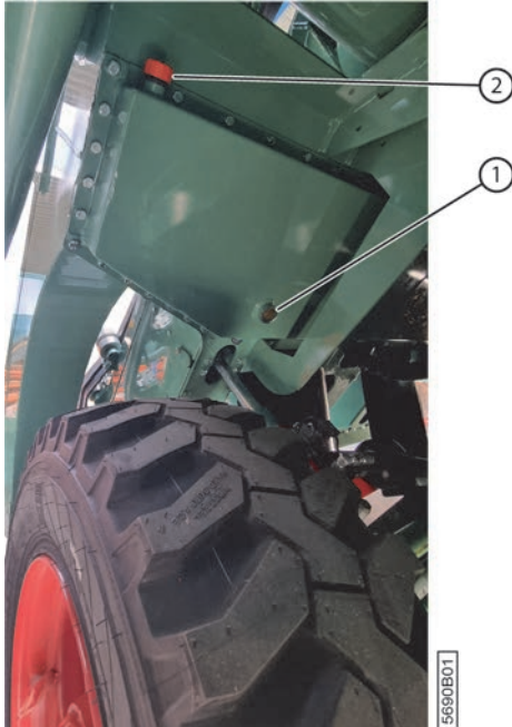
Fig. 108: Topping up the oil level in the gearbox for the picking element
