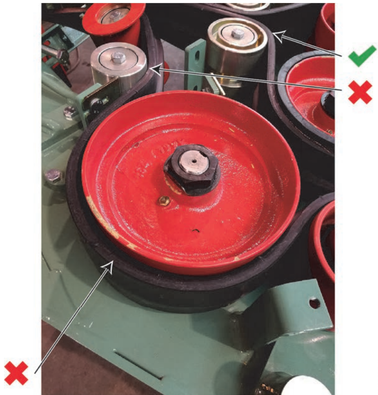
Fig. 137: Checking the alignment of the picking belts
