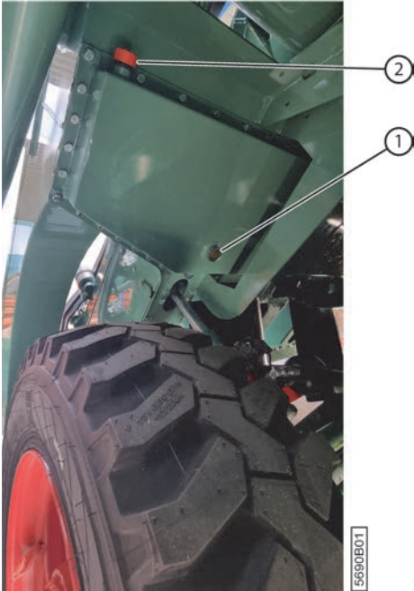
Fig. 107: Topping up the oil level in the gearbox for the picking element
