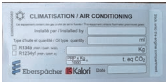
Fig. 159: The sticker with information about the air conditioning
