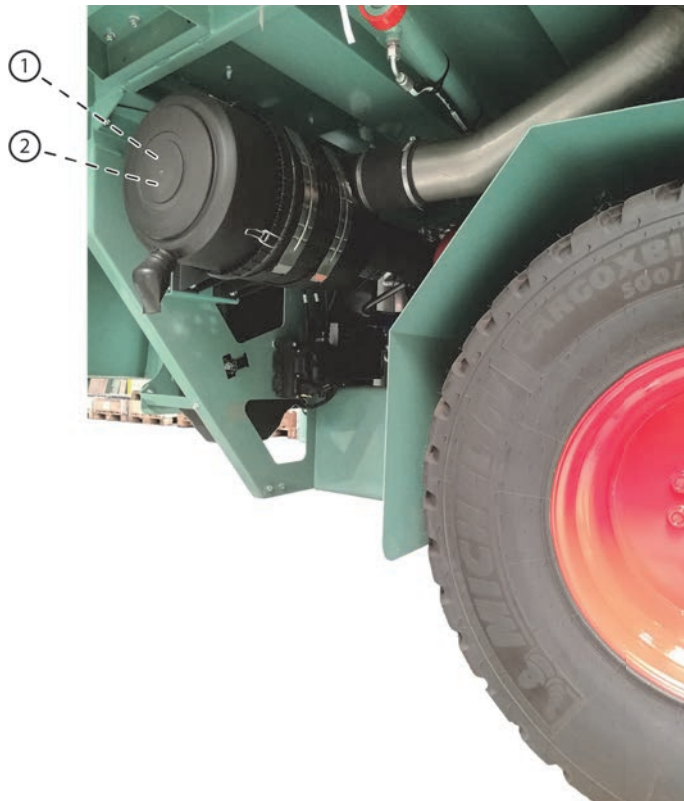
Fig. 183: Main element and safety element of air filter
