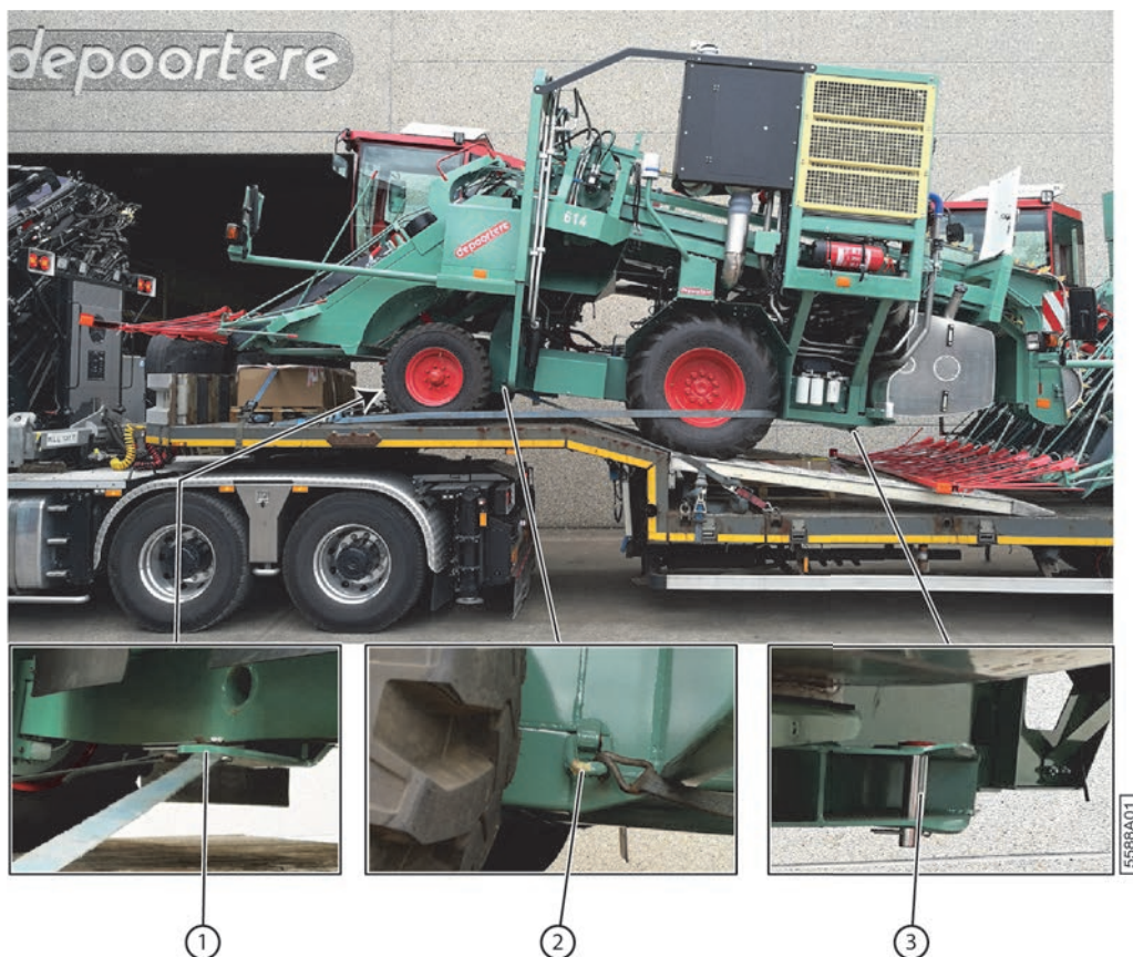
Fig. 46: Loading the machine onto the lorry
